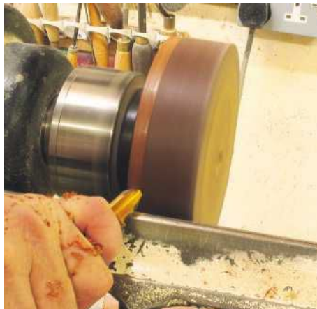
▲ Pic.5 The edge is done with the same tool but with a push cut. If you get the bevel in contact with the wood you should end up with a polished surface. Once again use your hand as a guide
